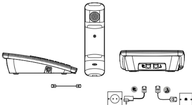
1. 将电话线插入座机后部标有
